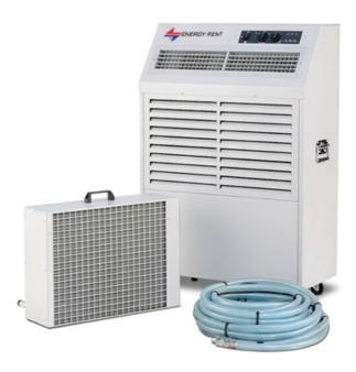
This compact unit consists of an indoor unit and an outdoor unit, which are connected by glycol-filled hoses quick connections A pump that ensures circulation is installed. The indoor unit has high and low pressure alarms as well as an automatic defrost system. The condenser heat is conducted through them glycol-filled hoses to the outdoor unit. KM 7 Cool is extremely flexible and is perfect for cooling server rooms, for use at events and in shops.
